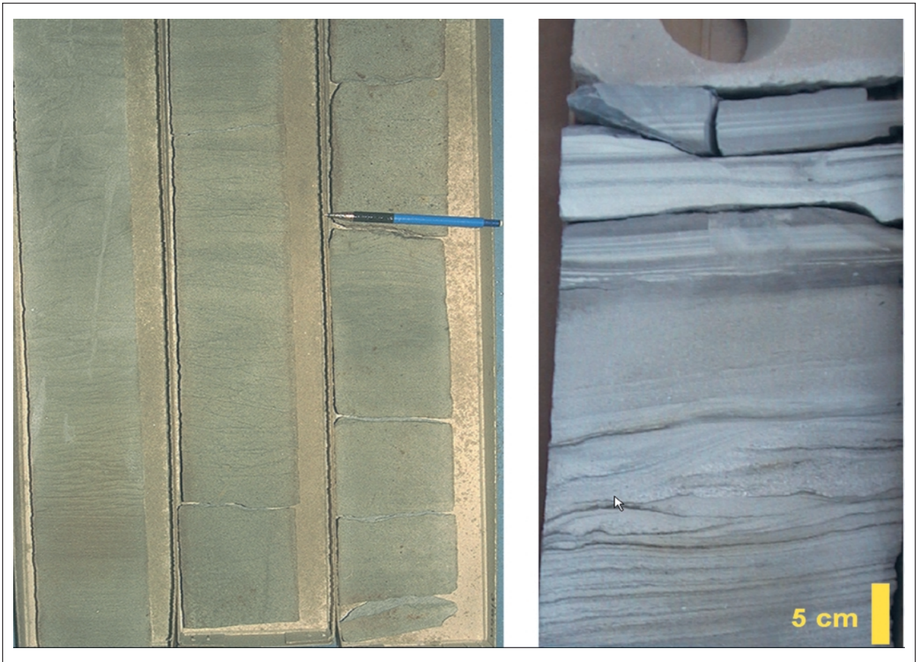
Fig.18. Core photos from facies association 3. A) 30/3A-1, T77C cycle: slope high-density turbidites with dish structures and long vertical burrows, 3186-3188 m. Note coarse basal layer above base of mass-flow indicated by pencil. B) 22/18-5, T77E cycle at around 8683 ft.: possible shallow marine indicators (double mud drapes near base of photo, wave/combined ripples in central lower part of photo) in a fine-grained interval between deposits otherwise interpreted as slope turbidites. The base of the succeeding mass-flow bed can be seen overlying laminated siltstones near the top of the photo.
