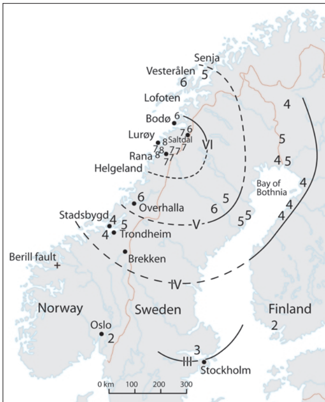
Fig. 1. Isoseismal map with intensity data points (redrawn from Muir Wood 1989) for the earthquake near Lurøy, Nordland on 31 August 1819. Average radius of perceptibility is about 800 km.
