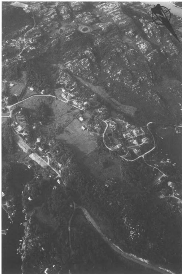
Fig. 15. N–S running fracture system near the tunnel entrance (the road leads to the tunnel just off the lower right corner of the picture), looking SSW.
