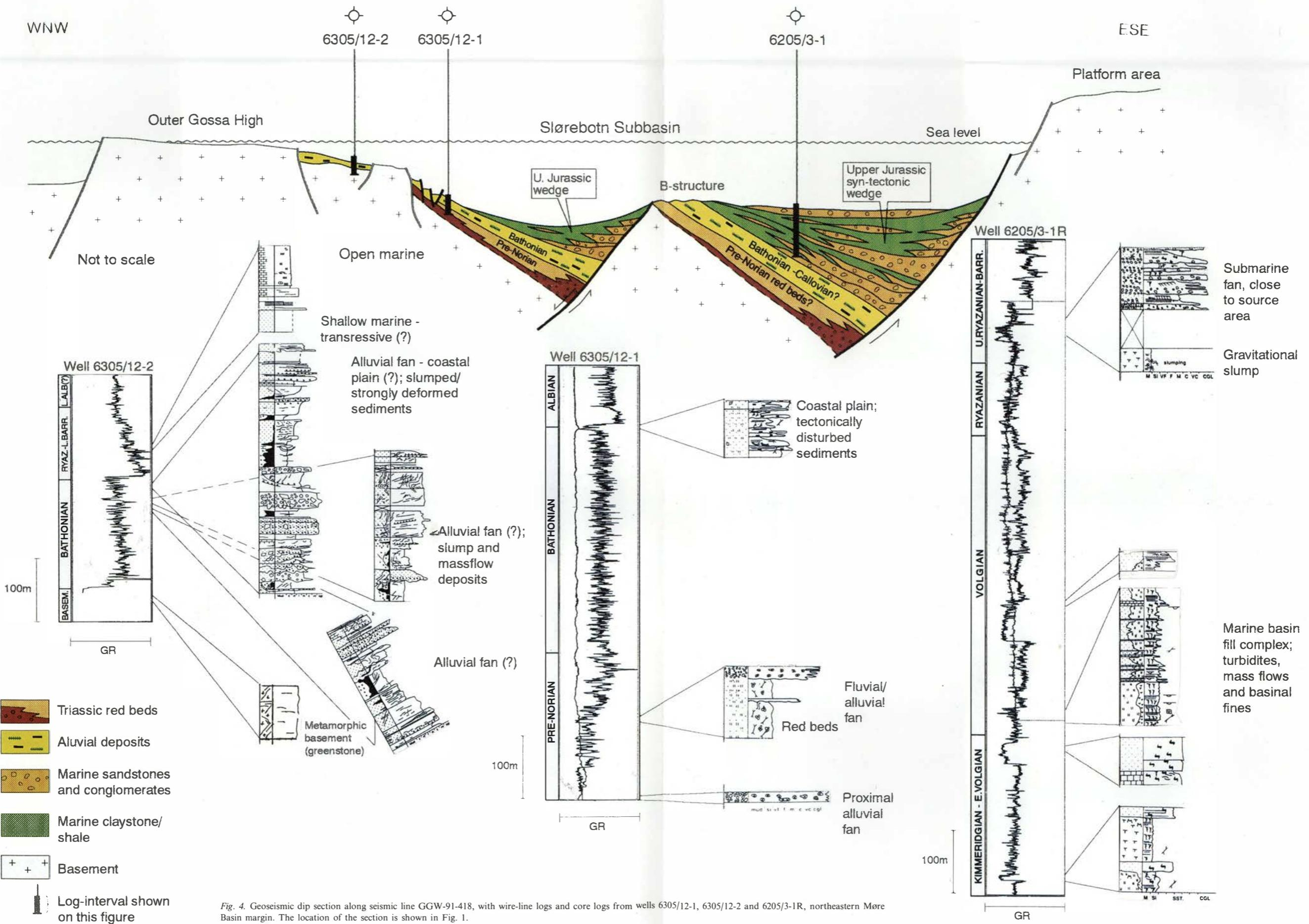
Fig. 4. Geoseismic dip section along seismic line GGW-91-418, with wire-line logs and core logs from wells 6305/12-1, 6305/12-2 and 6205/3-1R, northeastern More Basin margin. The location of the section is shown in Fig. 1.
