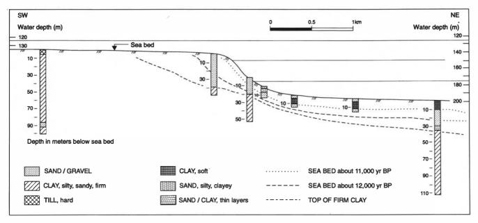
Fig. 2. Schematic section showing the conditions at the edge of the North Sea Plateau (location see Fig. 1). The soil drillings were done for the platform foundation at the Gullfaks Field (after Rokoengen et al. 1982).
