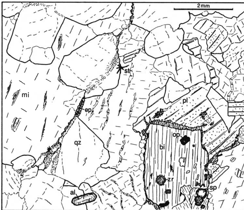
Fig. 2. Thin-section view of the Trysil 'Tricolor' granite. Granular texture, slightly disturbed by shear vein in left part of picture. See text for description. Minerals shown are: qz = quartz, mi = microcline, pl = plagioclase, bi = biotite, ep = epidote, sp = sphene, al = allanite, zr = zircon, st = stilpnomelane, op = opaques.
