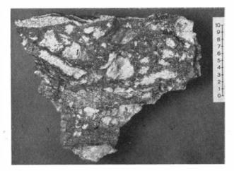
Figure 4. Feldspar porphyroblasts in a transformed gneiss (Sp. 542). The one RD orthoclase (see Figure 3) is marked by the number 1. The other prophyroblasts are microcline and a few plagioclases, scale in cm.
