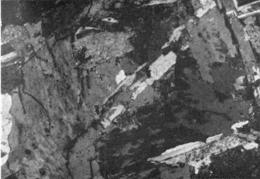
Figure 2. Primary plagioclase crystal replaced by albite component of an antiperthite, which also attacks an "antiperthite" unit (upper right). Crossed Nicols magnification 36\times . (Syenite: EAR 726).
