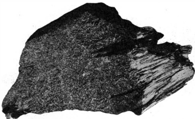
Fig. 8. Micaceous talc as cross-bladed vein in antigorite-serpentine. 2/3.
