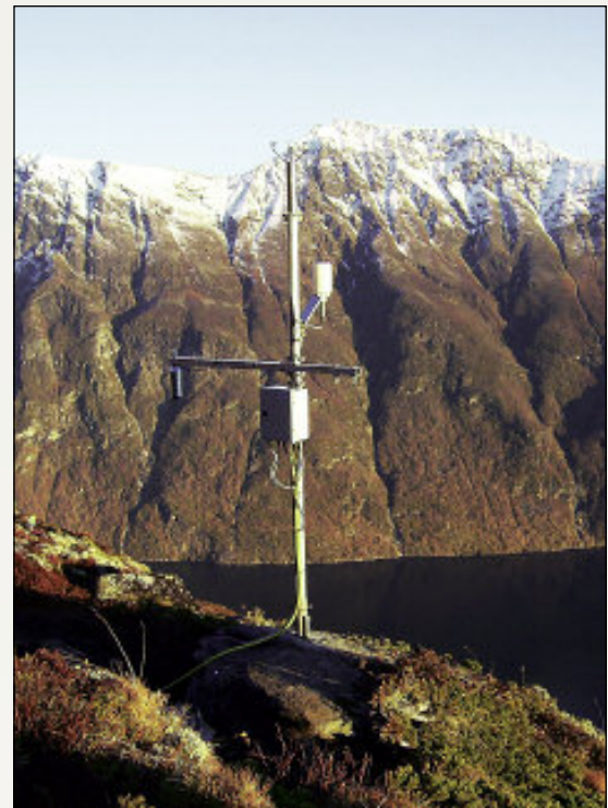
A climate monitoring station at Åkerneset records wind speed and direction, temperature, precipitation, solar radiation and snow depth. (Photo: L.H. Blikra)
