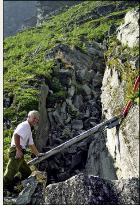
Crackmeters placed across fractures at Åkerneset provide continuous measurement of any expansion. (Photo: L.H. Blikra)
