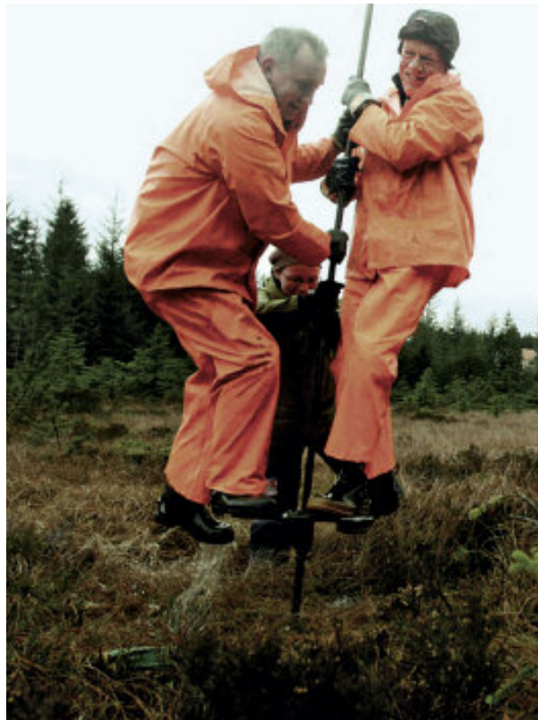
Researchers drilling in a bog on Askøy near Bergen for evidence of the 8,100 year-old Storegga slide tsunami. Studies such as this are important for predicting the potential consequences of future flood waves. (Photo: H. Hansen)
