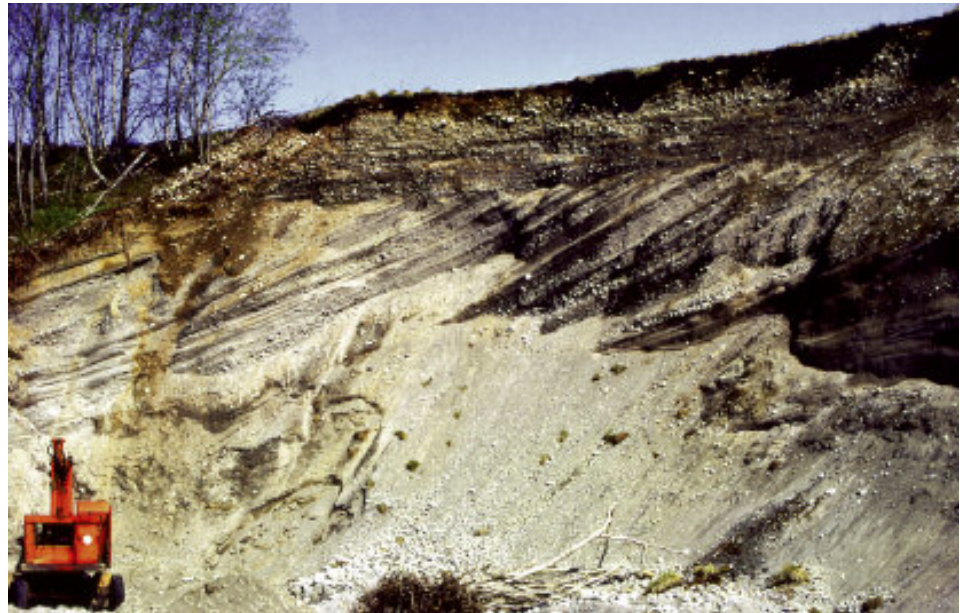
This gravel quarry at Sjøholt in the Sunnmøre region is typical of hundreds found at various locations along the Norwegian coast. It exhibits a meltwater delta with foreset beds dipping towards the sea and overlying almost horizontal topset beds deposited as the meltwater river flowed on top of its own foresets and prograded seaward. The boundary between the foreset and topset beds reflects the sea level at the time of formation; in this example about 60 m higher than today. (Photo J. Mangerud)
