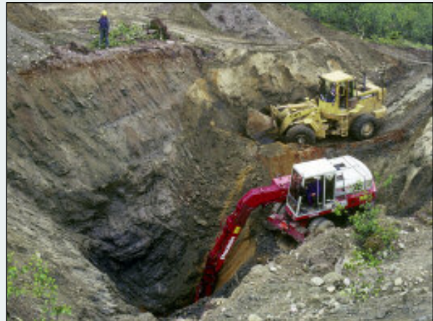
Searching for gold in the bedrock beneath a thick cover of till requires heavy-duty equipment. Sargejåk 1990. (Photo: M. Often)
