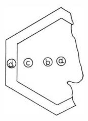
Fig. 1. Schematic diagram of zoning in beryl. Circled letters indicate sample location. Natural size.
